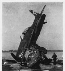
cocked into the wind and the pilot found that he didn't have sufficient control to straighten it out. He went off the runway on the right hand side at an angle of about 70° and tried without success to miss the truck which loomed up ahead by applying right brake and rudder.
