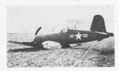
a center wing panel that is sprung and distorted, an engine that needs a major overhaul, and landing gear, flaps, and propeller that must be replaced.
