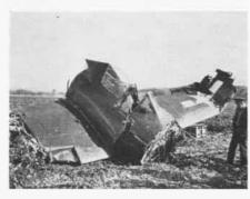
The picture above shows all that was left of an FR-1 after a spin accident during Field Carrier Landing Practice. The plane struck the ground in a steep left bank and cartwheeled on its nose. After shedding the tail section, aft jet engine, and forward engine, the cockpit section came to rest upright and facing 180 degrees from the original heading. The pilot was uninjured, because he had his shoulder harness and safety belt tight and locked.
