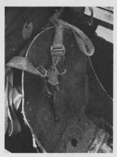
vent the ends of the shoulder harness adjusting straps from flapping around, they have been tied together, thus forming a loop across the pilot's chest.
