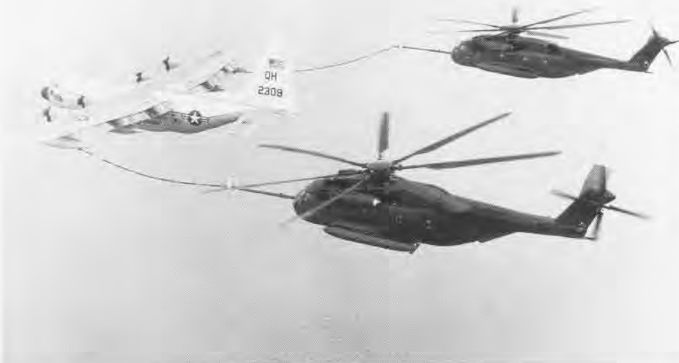
KC-130 Hercules mission: aerial refueling; transport for supplies, equipment and troops; ground refueling when other services are not available; and command and control of direct air support for ground forces.
