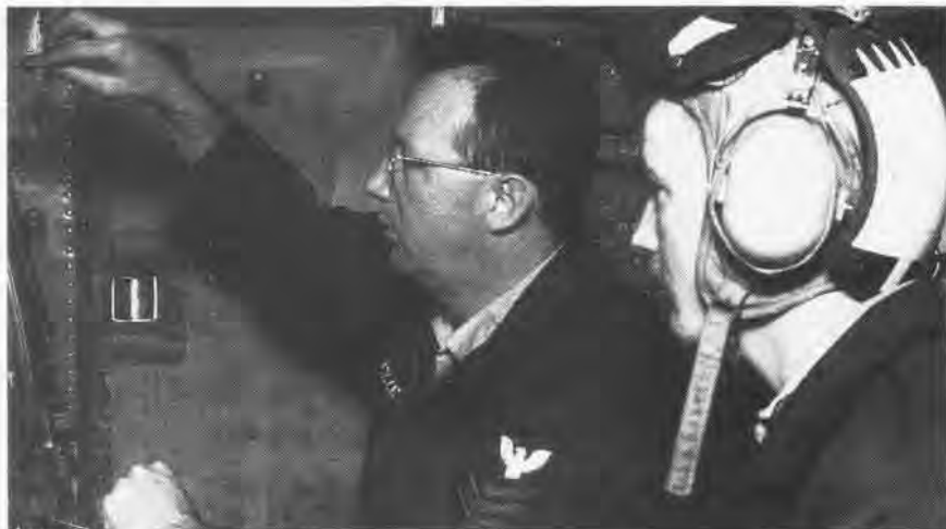
On-the-job training is key to learning the complicated systems ATs maintain. AT1 Robert Kelley demonstrates to ATAA Lindstedt how to install a main display unit on board an E-2C.
