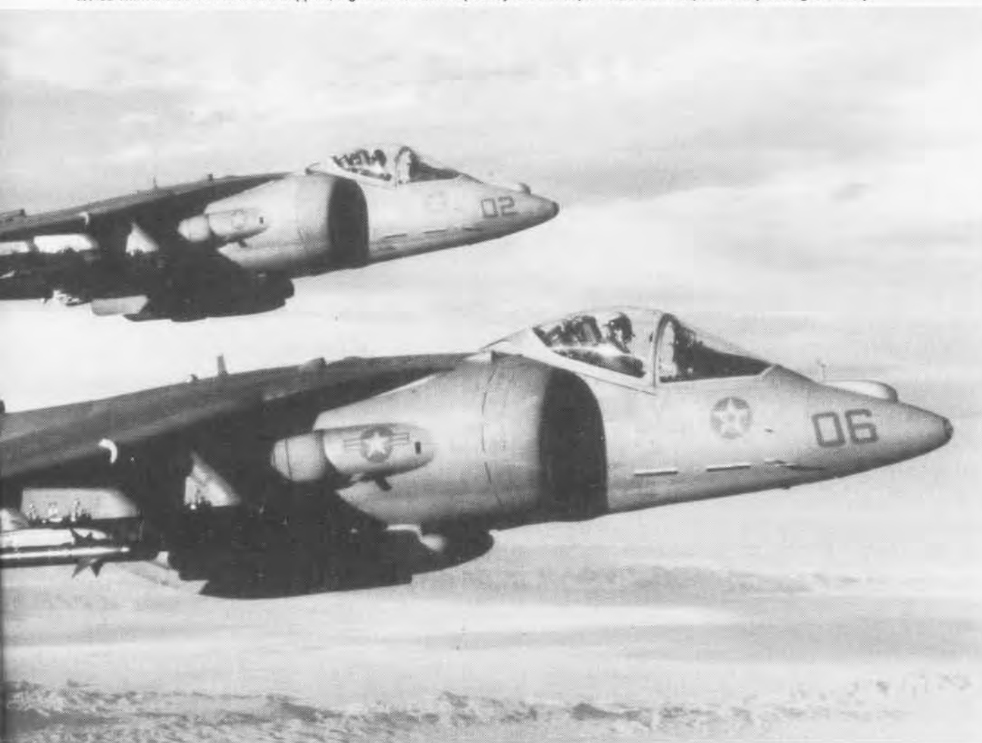
AV-8B Harrier mission: close-air support, night attack/radar capability and helicopter escort with expeditionary basing flexibility.
