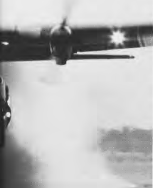
Smoke pours from the eight rockets strapped to Fat Albert during a jet-assisted takeoff.
