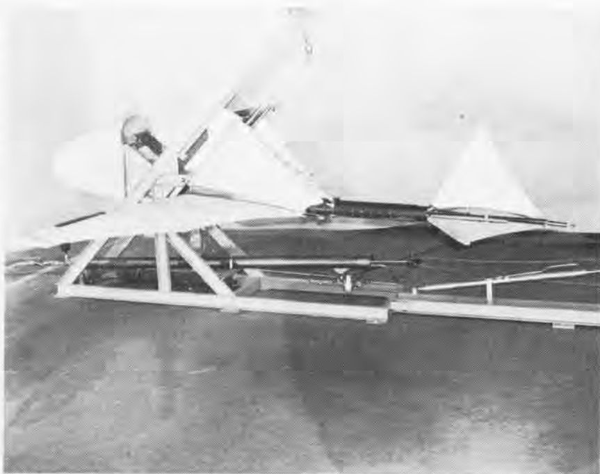
Flying ejection seat designed by Stratos Western Division utilizes the Princeton Sailing and an inflatable nose fairing to reduce drag and to protect the pilot. The craft also features a telescoping tail boom assembly and a turbofan engine.
