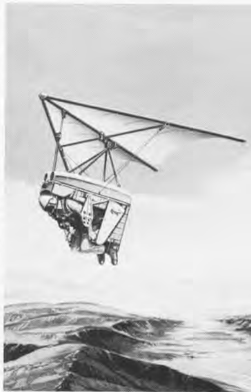
Parawing is being investigated by the Air Force. The Aerocab is deployed with the pilot facing down.
