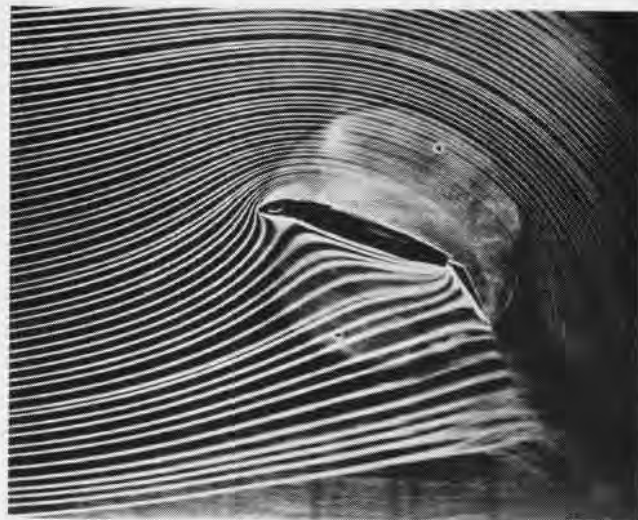
foil and angle of attack with supercirculation. Notice re-adherence of the flow to upper surface and also to the flap. Comparing the airflows in the parallel diagrams above, it is clear that lift increases tremendously; drag is nearly halved.
