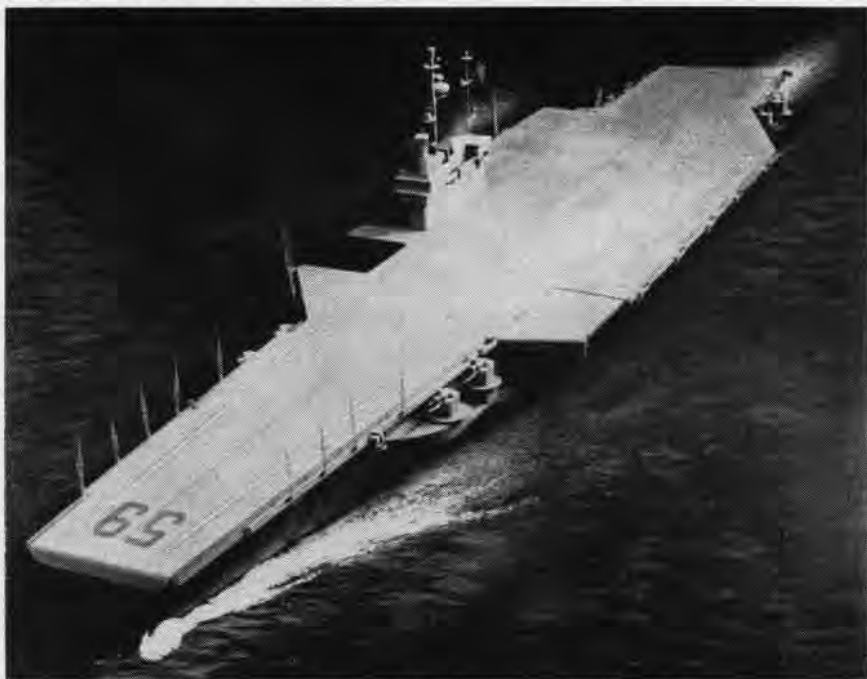
LATEST ARTIST conception of Forrestal Class carriers shows a fixed island, canted deck and four elevators. The catapults are indicated by white lines. The radio antennae can be swung to horizontal position during flight operations. The first of the class, the USS Forrestal , CVA-59, will be launched sometime this coming fall.
