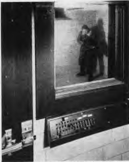
TESTING CAMERA IN -67 DEGREE ARCTIC ROOM
