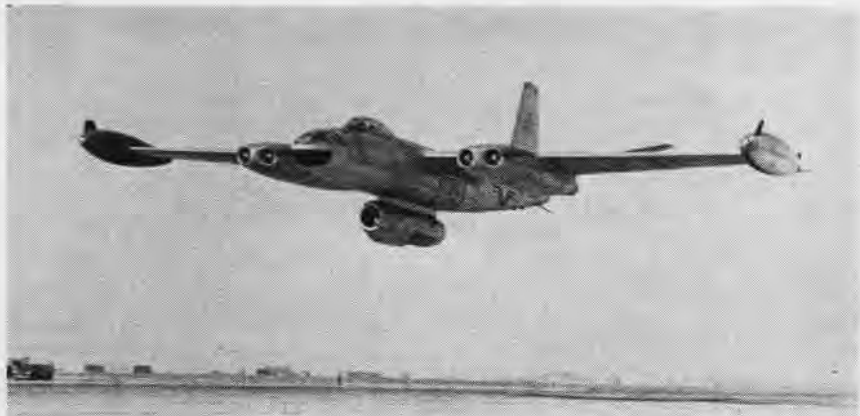
STRANGE-looking bomber is caused by an Allison 171 turbo-jet engine slung in a retractable pod built into the bomb bay of a B-45C bomber. The engine is being test flown from a flight test facility recently established by Allison at Edwards AFB.
