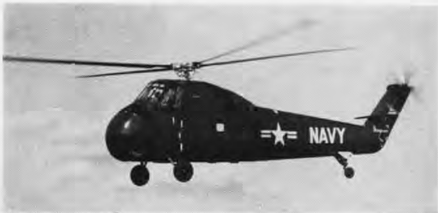
INTRODUCTION of dipping sonar is making the helicopter an active member of ASW team. Sikorsky's XHSS-1, which carries crew of four, joins the fleet next year.
