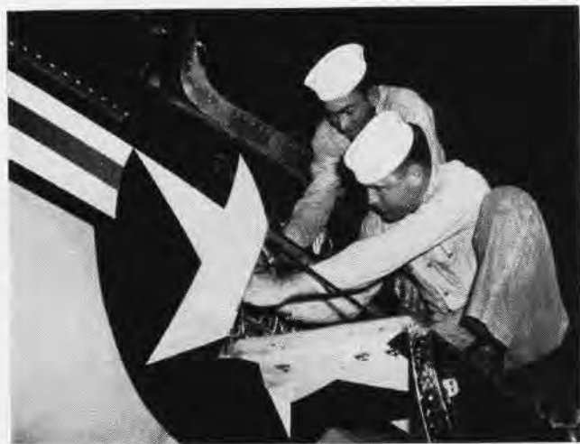
HYDRAULIC systems check is done by H. R. French, AM1, and J. H. Langston, AM1, through one of F7U-3's many access hatches.
