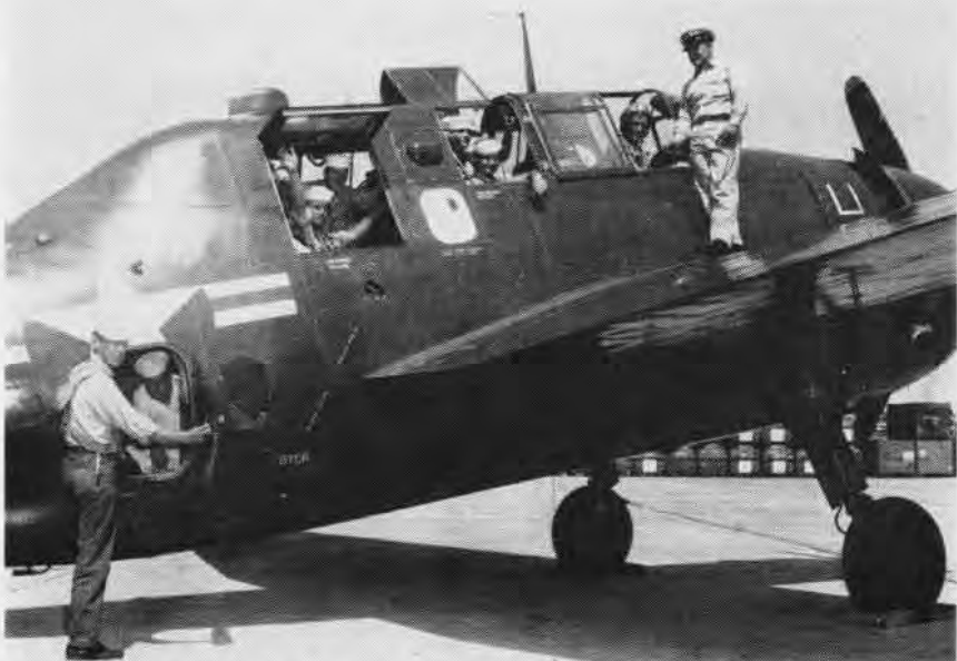
TBM-3R TRANSPORTS SEVEN MEN AND 2,000 LBS. OF GEAR TO AIRCRAFT CARRIERS AT SEA
