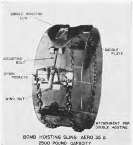
ADJUSTING BOLT AND WING NUT HANDLE SLACK
