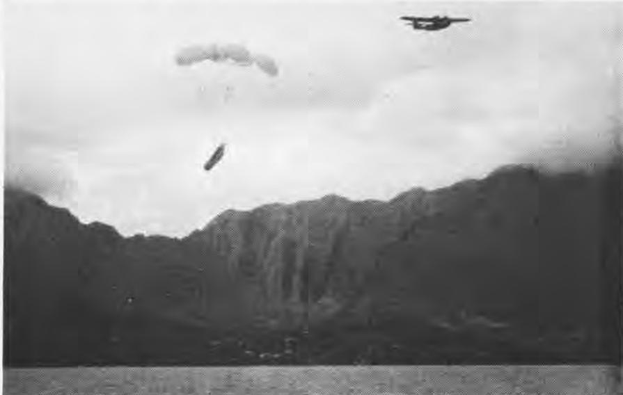
RELEASED FROM LOW ALTITUDE, BOAT IS LOWERED SAFELY TO THE WATER IN A FEW SECONDS
