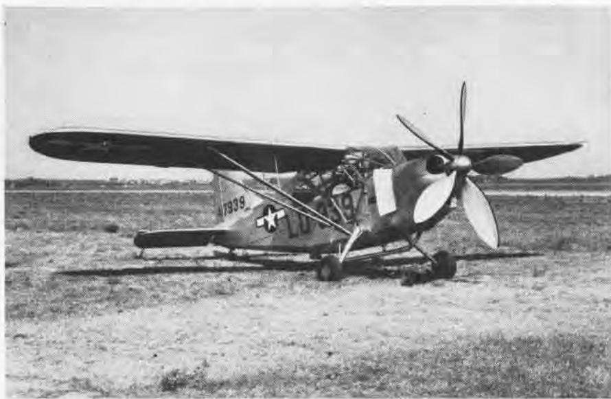
IN AN EFFORT to reduce the noise level of airplane engines, the National Advisory Committee for Aeronautics modified this Stinson L-5 by muffling the exhaust and installing a new type 5-blade propeller. The prop is driven at 1000 rpm by an engine geared-down to a ratio of 2.8 to 1. The reduction in tip speed reduces the noise level from 90 decibels to 66 decibels. This represents a reduction in noise pressure of more than 90 per cent.
