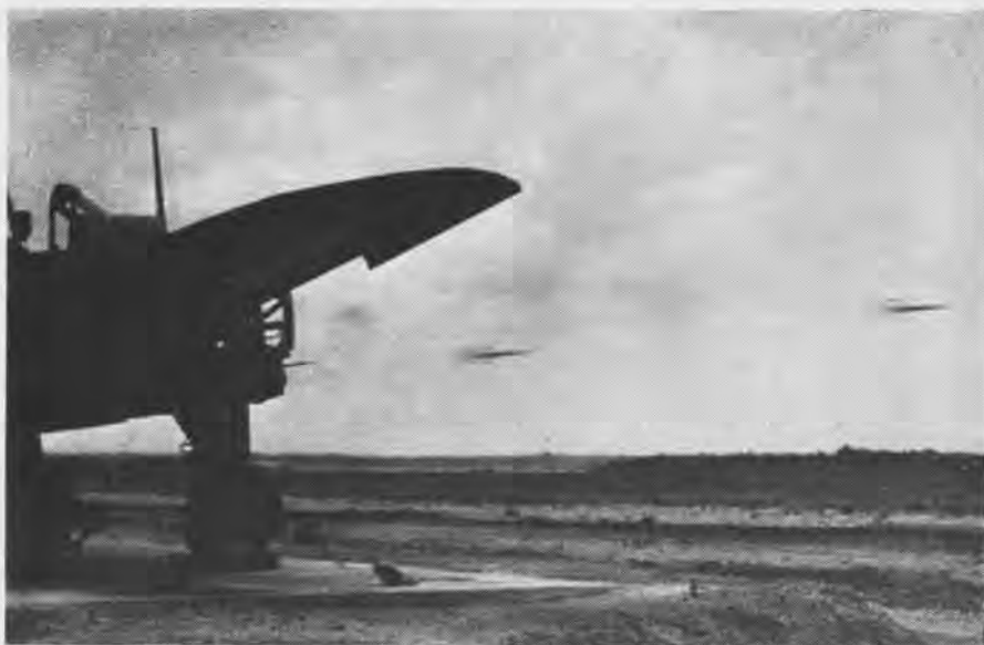
ZIPPING OFF the launching rails on a surveyed SB2C on the new rocket range at NAVAL AIR GUNNER'S SCHOOL, YELLOW WATER, may be seen two sub-caliber aircraft rockets in midair. Firing of these SCAR's is a new development of training naval personnel in rocket operations. Students at aviation ordnance officers school and advanced aviation ordnance school, before their graduation, have to assemble, load and fire a rocket
