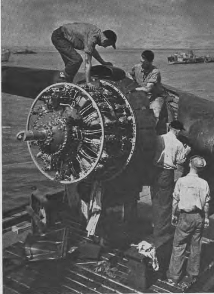
Aviation machinist's mates install starboard engine on a PBM after overhauling it aboard a seaplane tender. Smaller tender sends repair crews in rubber boats to do minor jobs on planes
