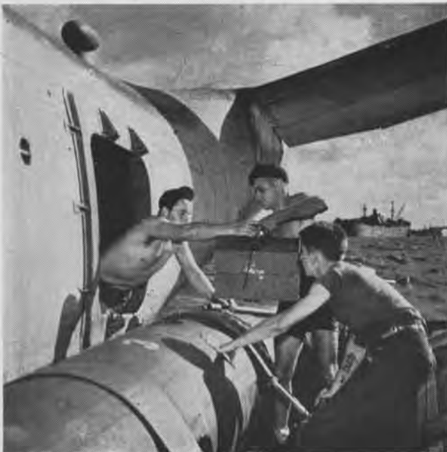
Seaplane tender crewmen in rubber boat pull alongside PBM at anchor, to make repairs. Only big tenders can hoist plane aboard
