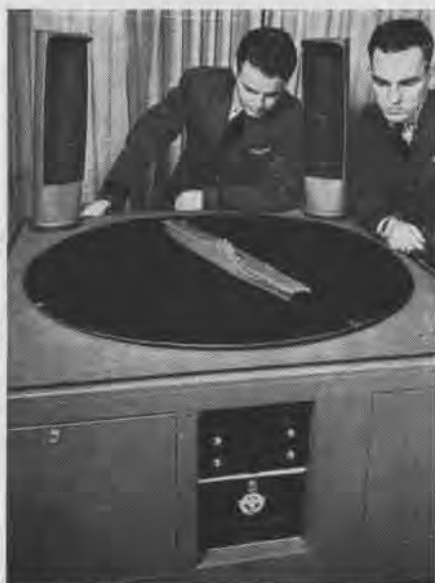
LIGHTED MODEL SIMULATES PITCH, ROLL
