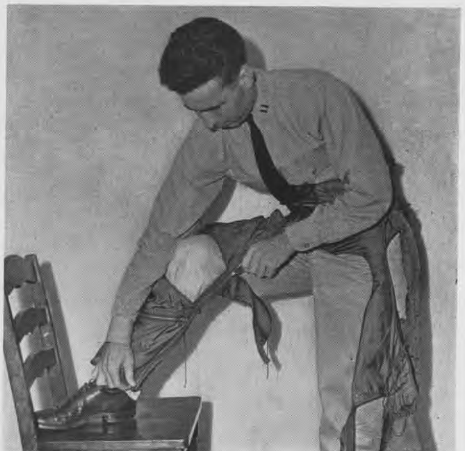
2 Like Types z-1 and -2, cutaway has 5 air bladders of plastic-impregnated cloth—2 over calves, 2 over thighs, and 1 over abdomen. Wearer puts suit on the right leg
