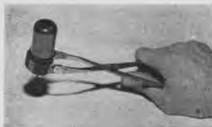
TOOL ELIMINATES RIVET HOLE ENLARGEMENT
