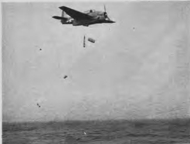
**Avenger** sweeps low as it releases AR-10 rescue assembly to survivors in water. Two shipwreck kits and raft, in that order, already have dropped from bomb bay. An outboard motor and fuel will follow. Entire assembly train is 280 yds. long
