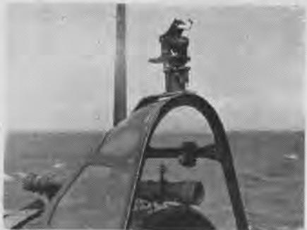
COMPASS IS FIRST INSTALLED ON A TEMPLATE
