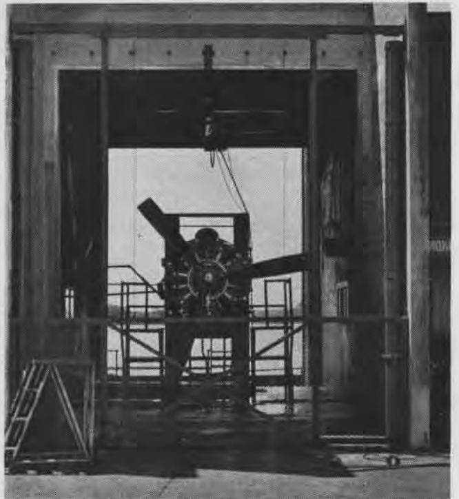
ENGINE DEFECTS ARE SOON FOUND BY A&R IN ITS OPEN AIR TEST CELLS
