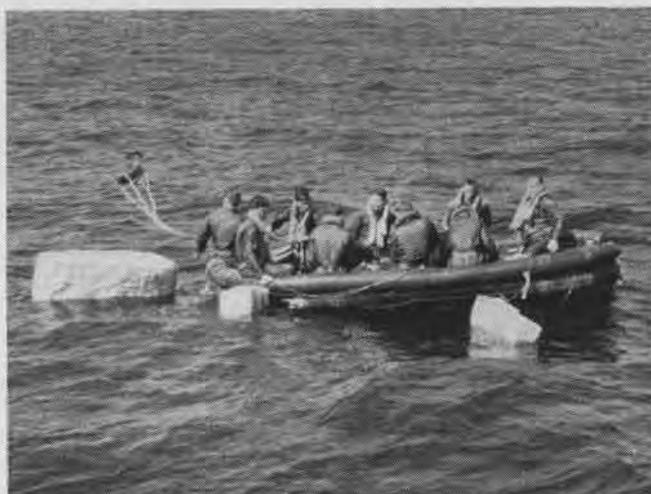
**Sea anchor** is thrown out as survivors ready raft for use. Two men on port side are inflating seats and rubber floor covering bilges, center and aft. Outboard motor, fuel and other AR-10 assembly units are hauled alongside life raft ready for stowing
