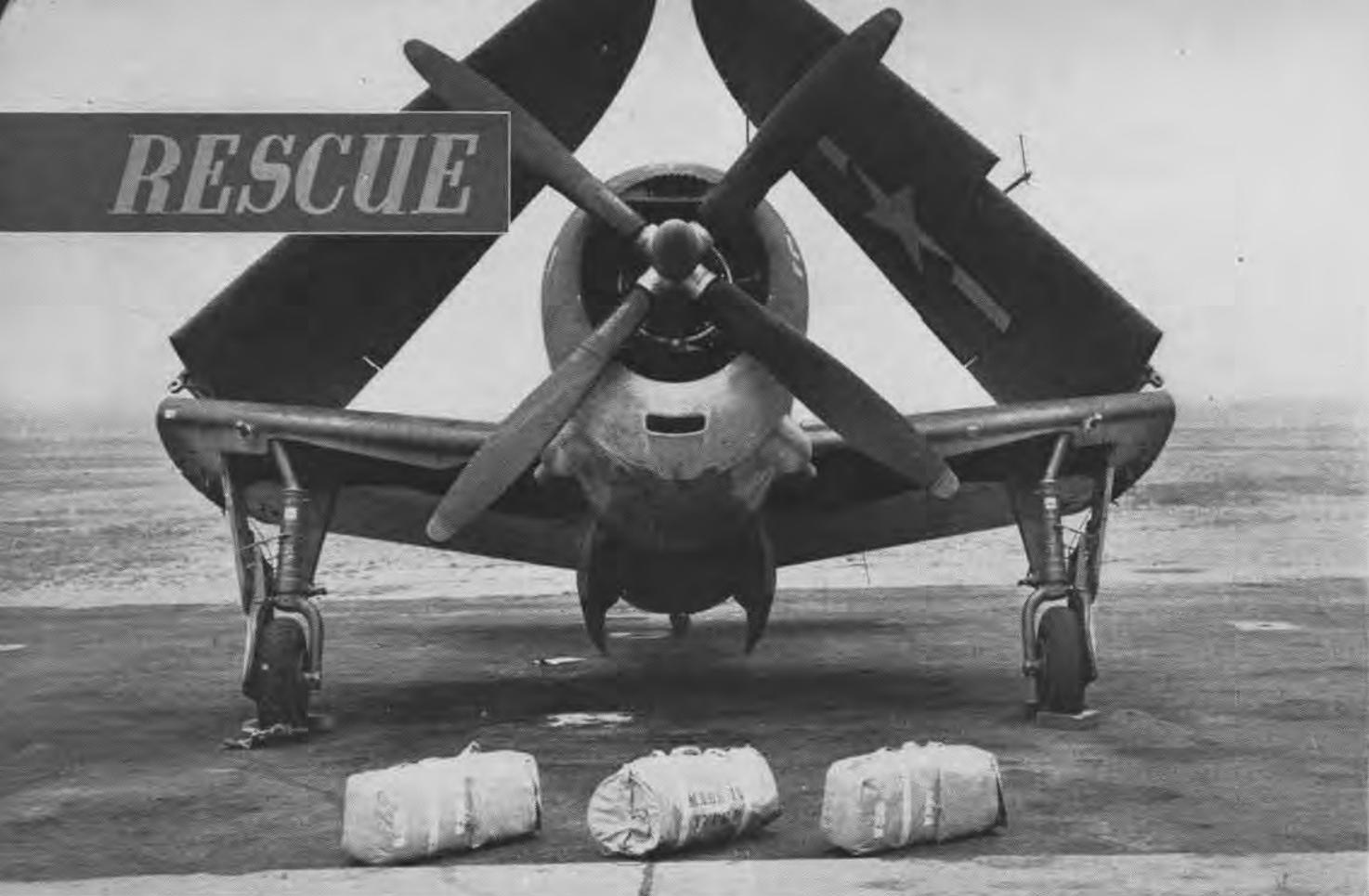
**Helldiver** with AR-4 rescue assembly ready for stowing. The gear is carried on the three internal bomb shackles of an SB2C. The entire AR-4 assembly is rigged in train for dropping and includes one pneumatic 4-man raft and two revised M-594 shipwreck kits
