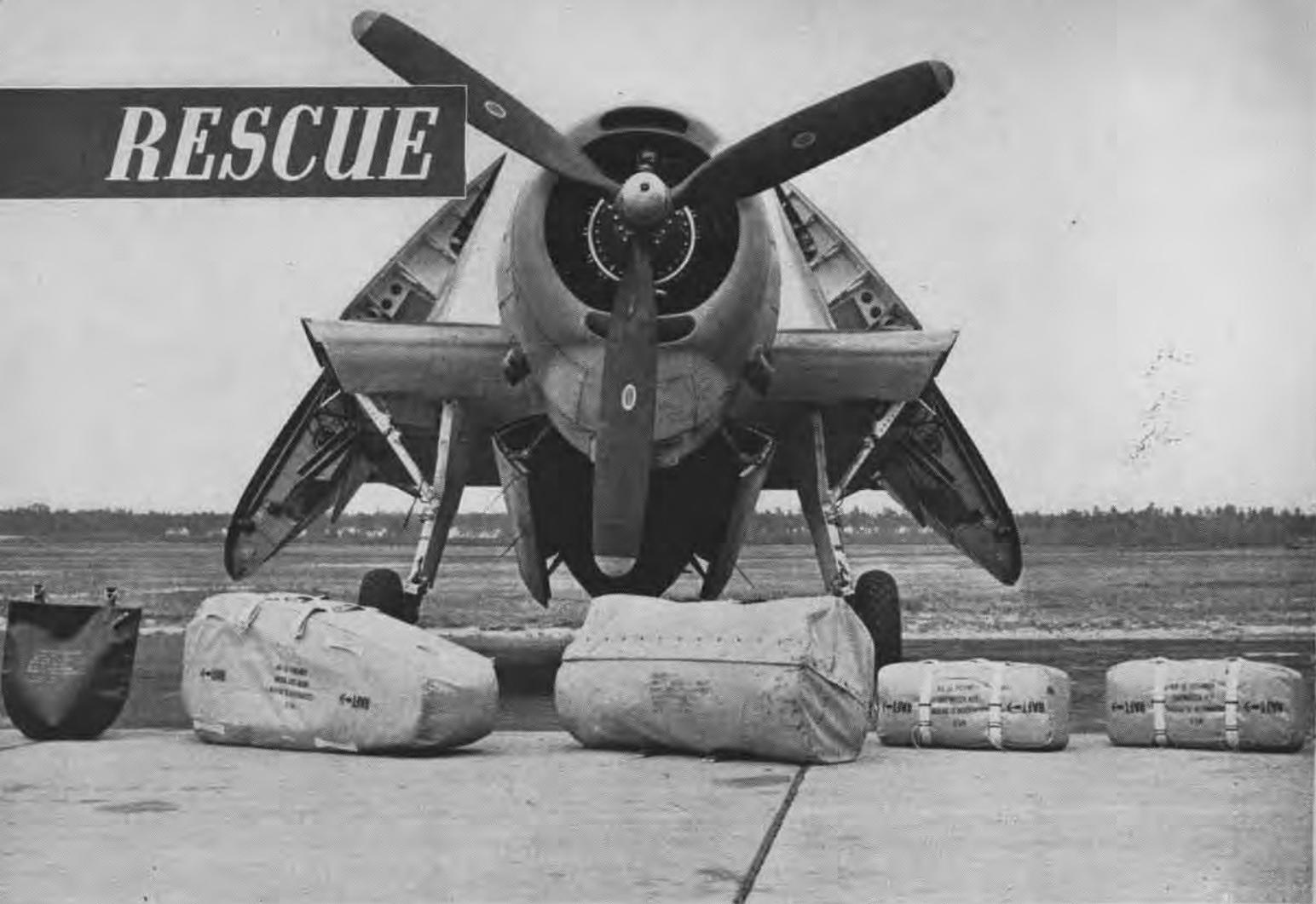
Shipwreck kits, pneumatic raft, outboard motor and fuel, in that order and properly rigged, fit snugly into Avenger bomb bay. An AR-10 assembly is dropped from 100 ft. elevation to survivors in sea below. Rescue units are connected by floating line
