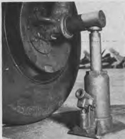
AXLE EXTENSION PERMITS FLAT TIRE REPAIRS
