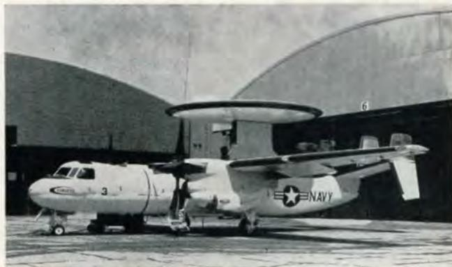
retrieve badly-needed repaired items. The E-2A Hawkeye (R) is shown with AN/APS-111 radar and AN/APA-164 rotodome installed. This new system provides improved definition of approaching aircraft and reduction of ground clutter. The Hawkeye will make its first appearance with the Seventh Fleet by the end of this calendar year.
