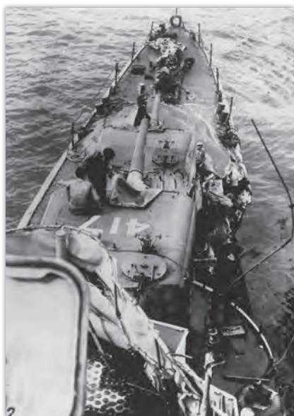
A starboard view of the destroyer Morris (DD-417) shows damage received from a kamikaze on 6 April 1945, while operating off Kerama Retto, c. June 1945. (NHHHC, NH 94448)
