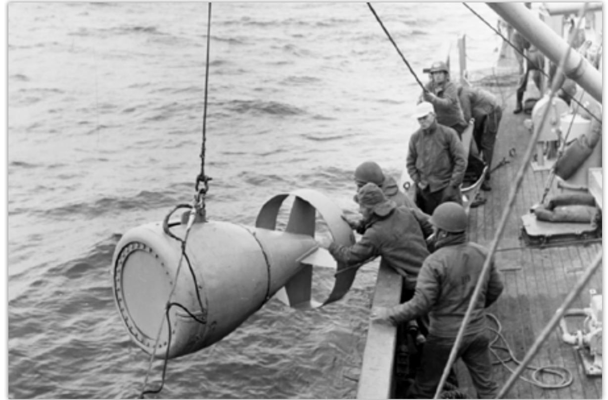
Sailors on board minesweeper Mockingbird (AMS-27) deploy an acoustic hammer box to locate the magnetic-influence mines discovered during sweeping operations off Wonsan. This type of mine disrupted the final sweep of the channel, forcing postponement of the landing. (NA 80-G-422164)
