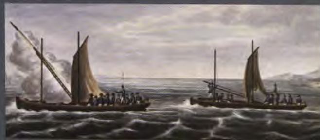
Top, William Congreve. Bottom, two launches throwing rockets: the lead boat is in the act of firing—the crew retires into the stern sheets and a marine artilleryman discharges a rocket by a trigger-line, leading aft; in the second boat the artillerymen are loading a rocket by lowering the frame.
