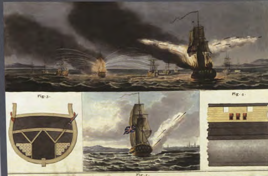
Above, Congreve adapted rockets to any ship by using scuttles or openings on the side of the hull. Left, this Congreve rocket, with part of the original stick still attached, was found in Stonington, Connecticut, after the British bombarded that town in August 1814.
