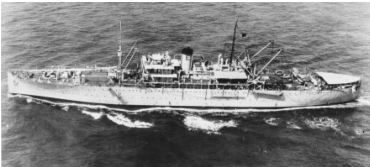
Wright, AV1 with seaplane on board; the first U.S. Naval vessel especially fitted as an aircraft tender 1053778
