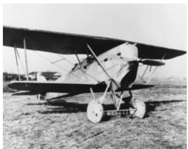
FB-5 fitted for longitudinal arresting wires 458533
