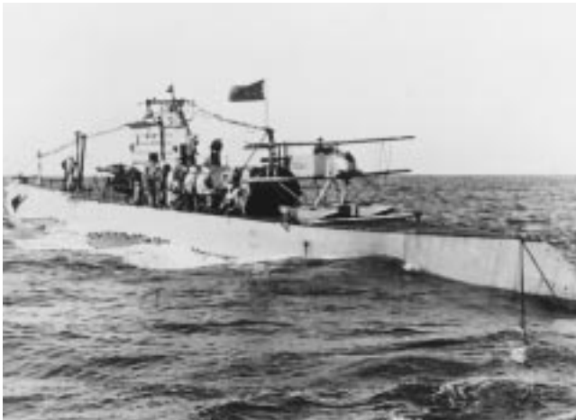
S-1 demonstrates the feasibility of operating aircraft from submarines in tests with XS-2 seaplane, 1926 1053777
