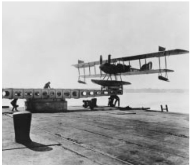
Aircraft were launched from capital ships by turntable catapult, shown on a pier at NAF with an N-9 428435
