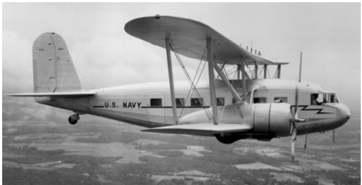
The R4C-1 Condor was used as a transport by the Navy, AN-32600.
