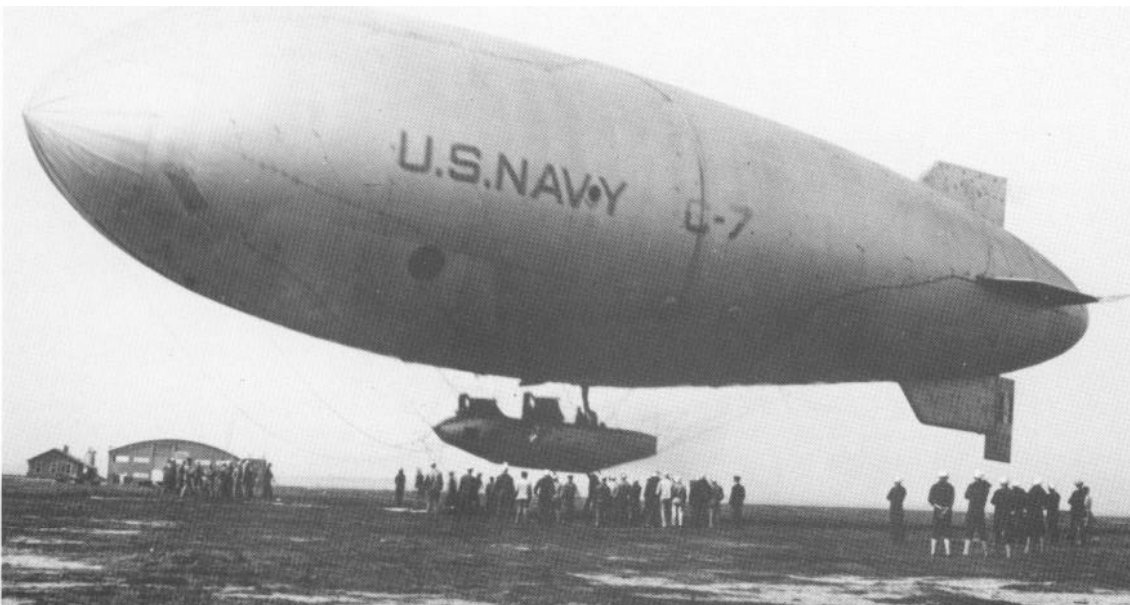
The C-class set many "firsts" in Naval Aviation. This particular airship, the C-7, was the first airship to be inflated with helium.
