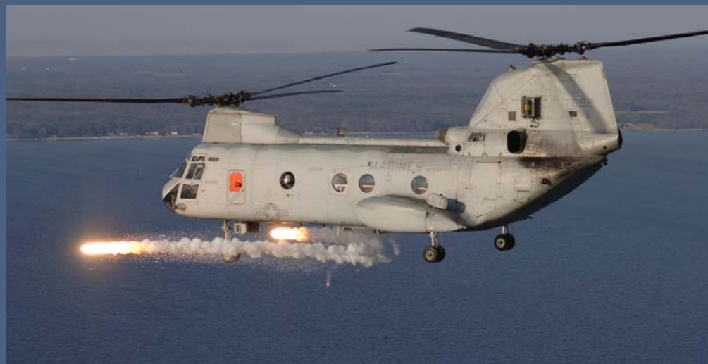
Left, a modified chaff and flare dispensing system is tested on a CH-46E Sea Knight at NAS Patuxent River, Md., on 22 February. Background, HX-21 conducted the first firing of AGM-114 Hellfire missiles from an MH-60S on 30 January, also at Pax. Photo by Kurt Lengfield.
