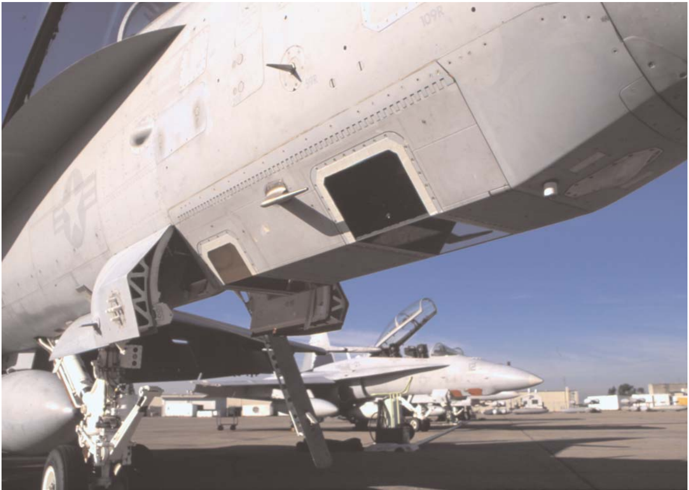
Previous page, Green Knights F/A-18D Hornets perform a flight breakup during exercises over the southern California desert. Above, although the ATARS replaces the Hornet's 20mm cannon, the aircraft's expanded reconnaissance capabilities have proven valuable to Marines on the ground. Right, ATARS and non-ATARS-equipped Hornets are purposely grouped together in section flight in order to exploit the capabilities of each aircraft.
