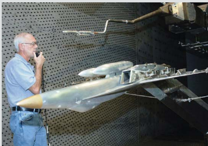
A HARM model is suspended above a Super Hornet model during wind tunnel testing at Arnold AFB, Tenn., as machinist Carey Wofford relays information to test personnel. Photo by David Housch.
