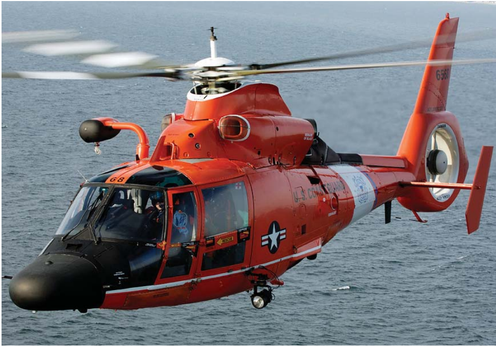
Above, a re-engined HH-65C flies seaward out of CGAS Atlantic City, N.J., during a routine maritime mission. The more powerful Charlie has been praised by air crew members and ground personnel for its versatility and easy maintenance. Photo by Dan Megna. Right, AMT2 Jason Taylor conducts preflight checks on the engine of an HH-65C at CGAS Houston, Texas. Photo by PA2 Adam Eggers.
