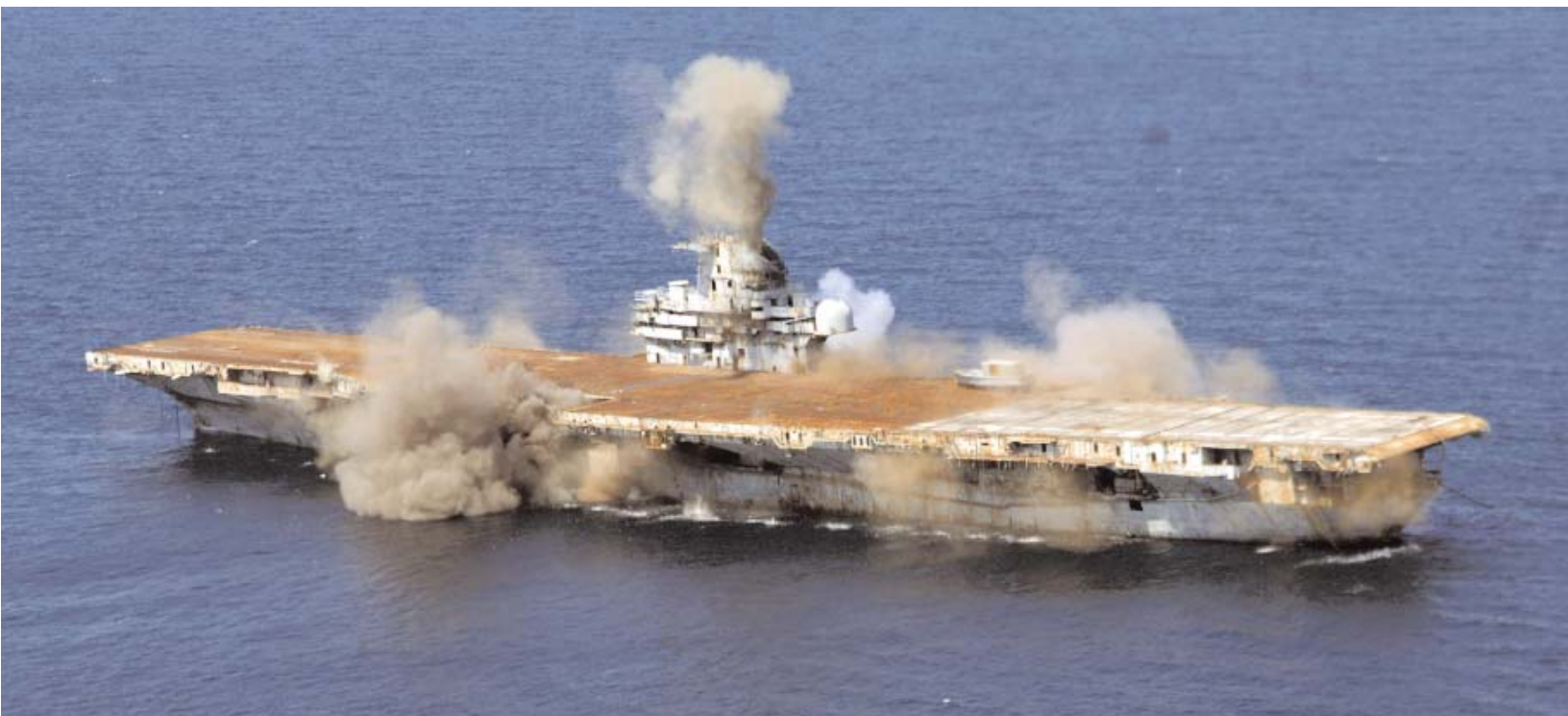
The ex-Oriskany , which served the fleet for more than 25 years in places like Korea, Vietnam, and the Mediterranean Sea, was sunk on 17 May off the coast of Pensacola, Fla., to form an artificial reef. The 888-foot, 32,000-ton vessel took about 37 minutes to sink 212 feet below the surface after strategically placed explosives were detonated throughout the ship, above. As an artificial reef, the ship will now benefit marine life, sport fishing, and recreational diving off the Florida panhandle. Photo by MC2 Jeffrey P. Kraus.
