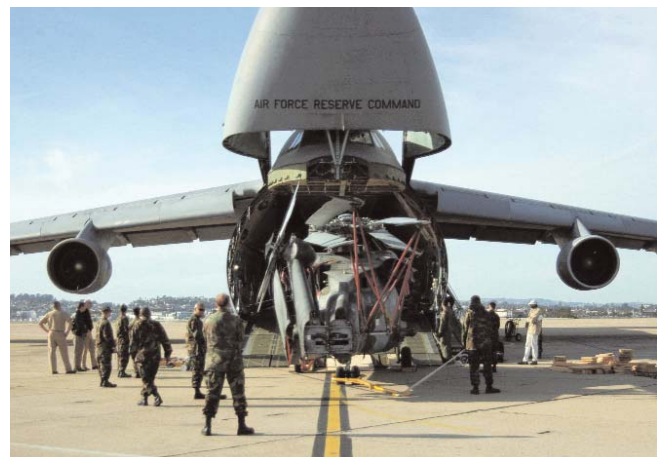
HS-10 sailors oversee the loading of squadron helicopters on a C-5 Galaxy prior to deployment.
