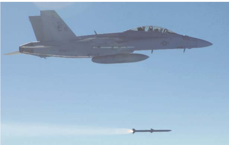
An F/A-18F Super Hornet launches an advanced medium-range air-to-air missile during developmental testing for the advanced electronically scanned array system at NAWS Point Mugu, Calif., on 19 October 2005.
