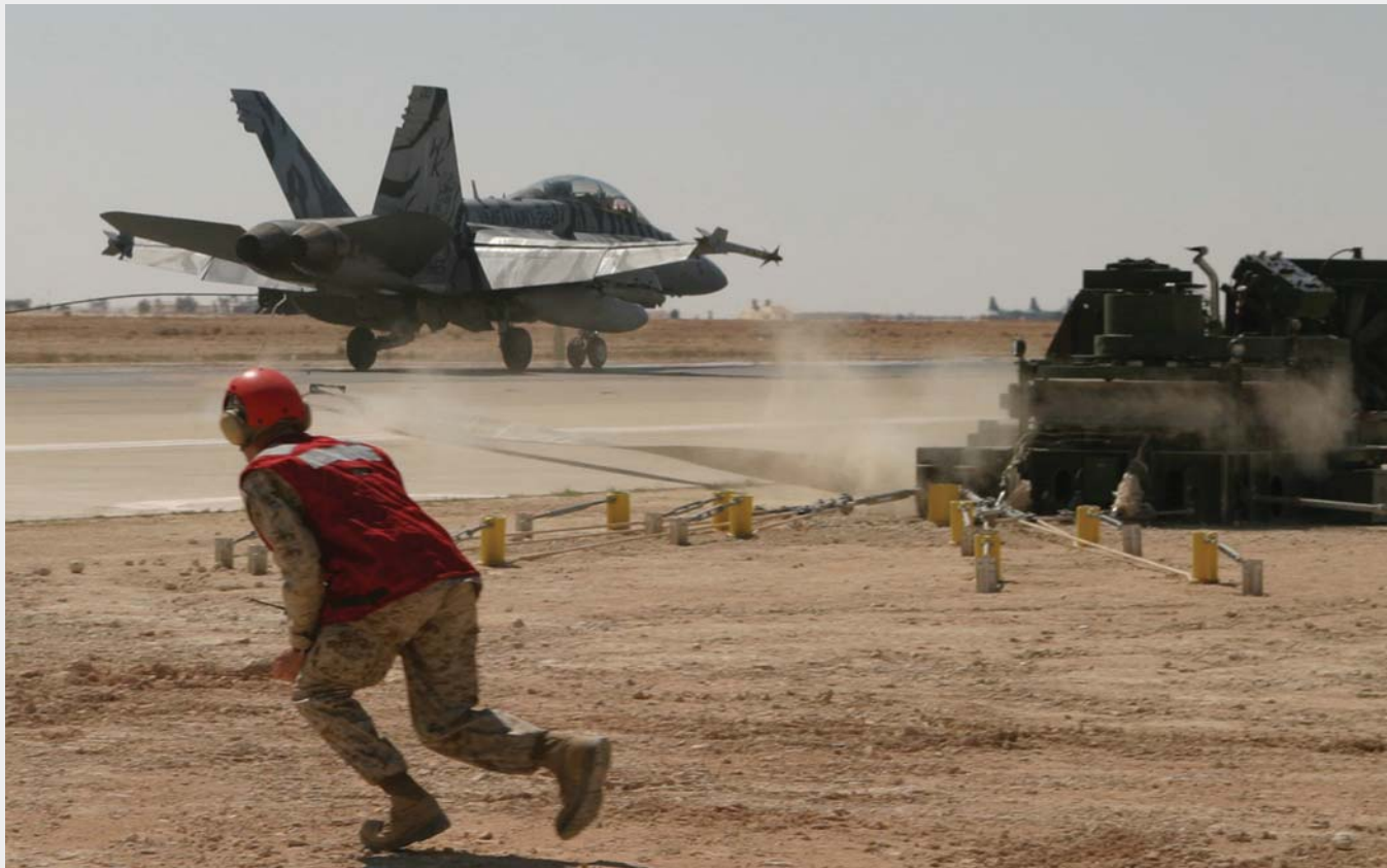
A Marine All Weather Fighter Attack Squadron 224 F/A-18D Hornet catches the wire of the expeditionary arresting gear at Al Asad, Iraq, on 26 March. Expeditionary airfield technician Sgt. James S. Happle runs to check that both sides of the gear are functioning properly.
