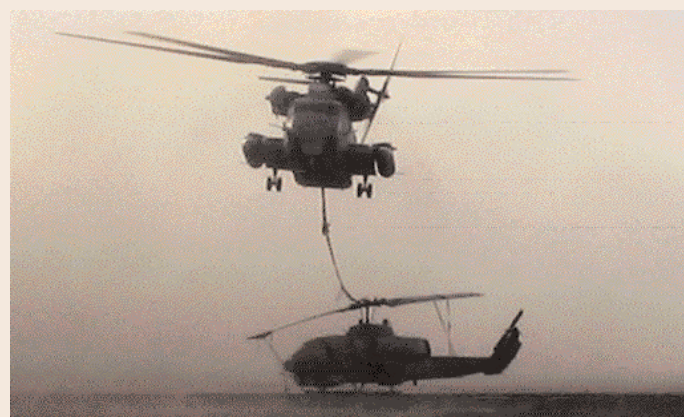
An HMH-361 CH-53E lowers a battle damaged AH-1W of HMLA-169 at Al Taqaddum, Iraq.
