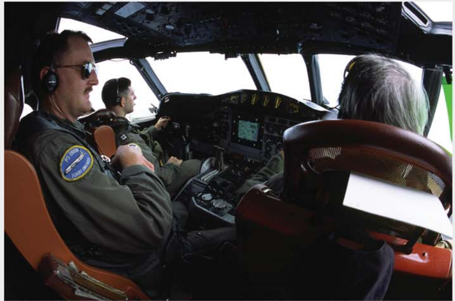
Left, an NP-3D returns from a training mission. The school utilizes two of these specially configured aircraft in the systems syllabus. Above, the NP-3D's flight deck includes a unique center display, containing the FLIR, radar, and navigation tools. Below, a student checks a setting at the navigation assessment station.
