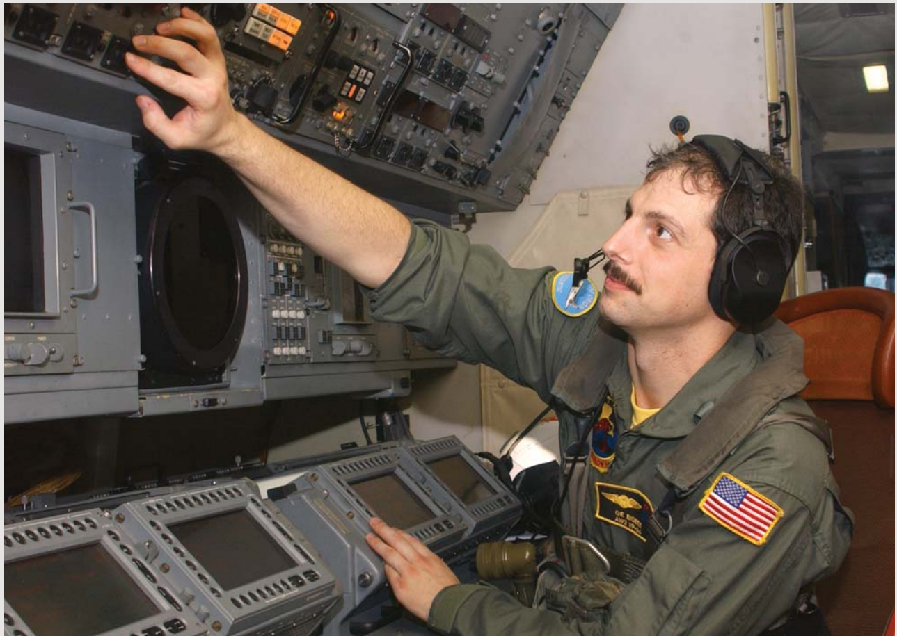
AW2 Glenn E. Bigbee of VP-94 performs a preflight check on the antisubmarine acoustics system aboard a P-3 Orion.
