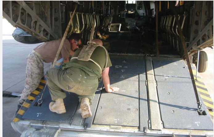
Marines of HMH-461 install the Ballistic Protection System on a squadron CH-53E Super Stallion. The system adds approximately 1,500 pounds to the helo's weight.
