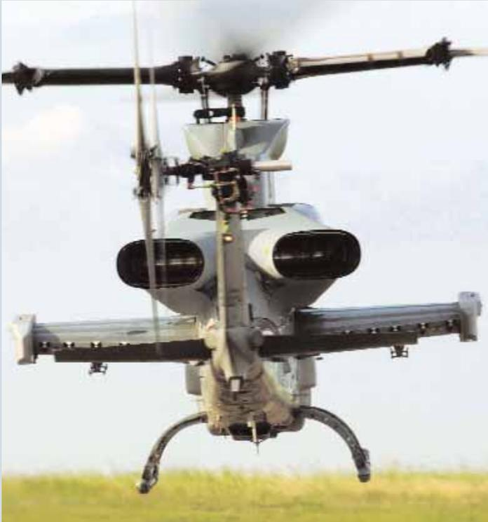
the tail boom. Designed for the AH-1Z Super Cobra and UH-1Y “Huey” upgrades currently in developmental testing, the turned exhaust will also begin testing for the fleet AH-1W Super Cobra in October.
