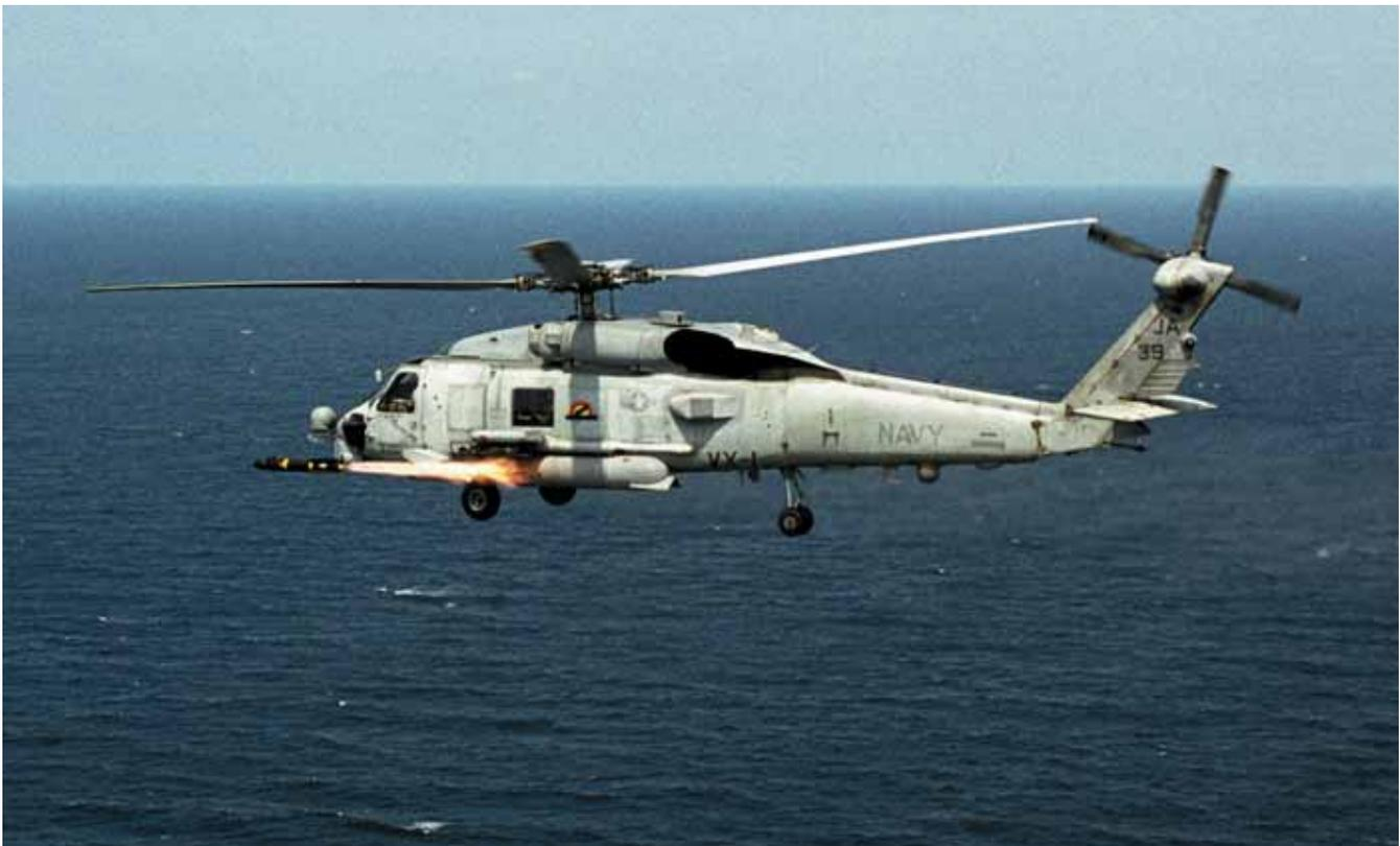
**Above, VX-1 fires an AGM-114M Hellfire missile from an SH-60B Seahawk for the first time, over the Chesapeake Bay. Right, a crew from VX-1 tests the vertical replenishment capabilities of the Navy's newest helicopter, the MH-60R.**
