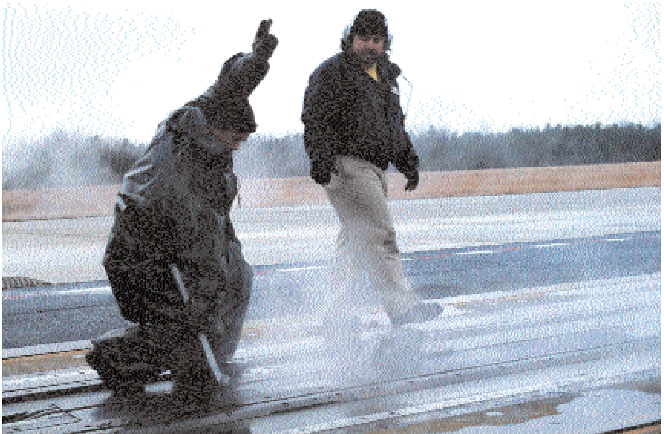
Right, Sailors work beneath the elevated platform of the 1959-vintage catapult in use at NAVAIR Lakehurst. It has survived many modifications to keep pace with the changing needs of aircraft carriers. Below, Test Department personnel “topside” ensure the catapult’s mechanisms are safe for the next no-load launch.
