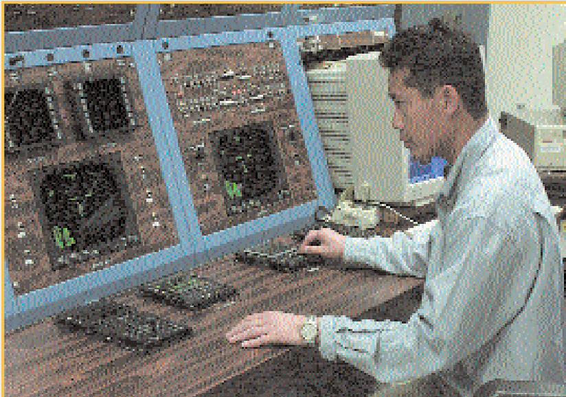
Above, Chu Fang of NADEP North Island's research and engineering department tests the global positioning system and armament software of an SH-60 Seahawk . Above right, NADEP North Island is the only Navy facility performing depot-level maintenance on the LM2500 turbine engine, which powers many Navy surface vessels. Right, the depot is capable of manufacturing wire bundles and electrical components. Below, AT2(AW) Cesar Decena (seated) and AT2 Stephen Applebaum perform a series of tests in the depot's Fleet Calibration Laboratory.
