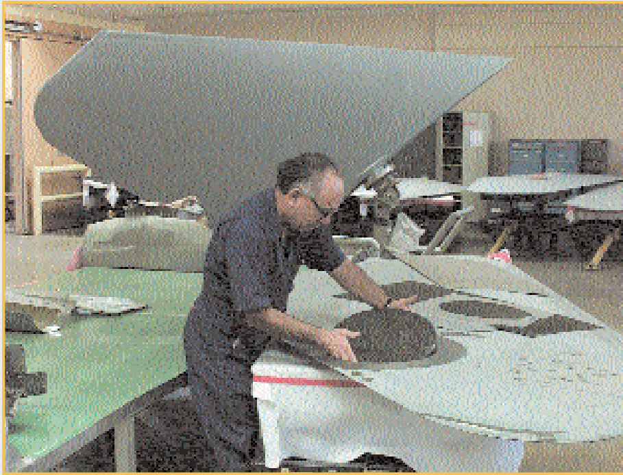
Left, NADEP North Island artisan John Ruiz carefully tests the fit of a section of honeycomb in an F/A-18 Hornet stabilator. The depot was the first DOD facility to repair aircraft components made of or using composite materials. Below, Leon Boykin, one of the more than 3,000 civilian employees of NADEP North Island, performs fiberglass repairs on an S-3 Viking nose cone. While the majority of NADEP artisans are veterans of military maintenance operations, only about 70 are active-duty Navy personnel.
