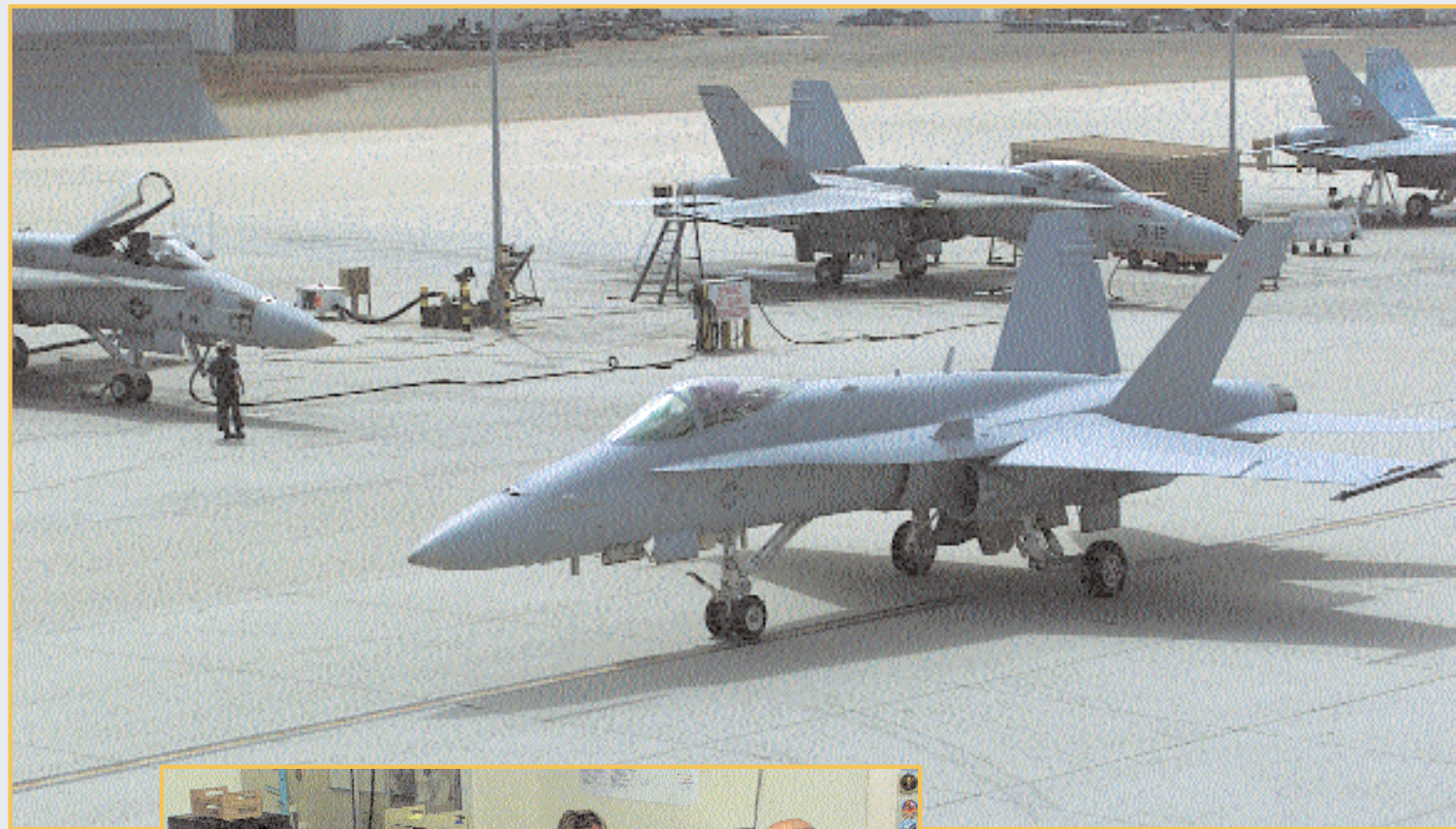
Above, an F/A-18 Hornet taxis from NADEP North Island's test line for a check flight. Depot pilots, sometimes assisted by squadron pilots and aircrew, fly check flights on all aircraft before they are returned to the fleet. Left, maintenance control center personnel at NADEP North Island brief depot pilots on the status of aircraft before check flights.
