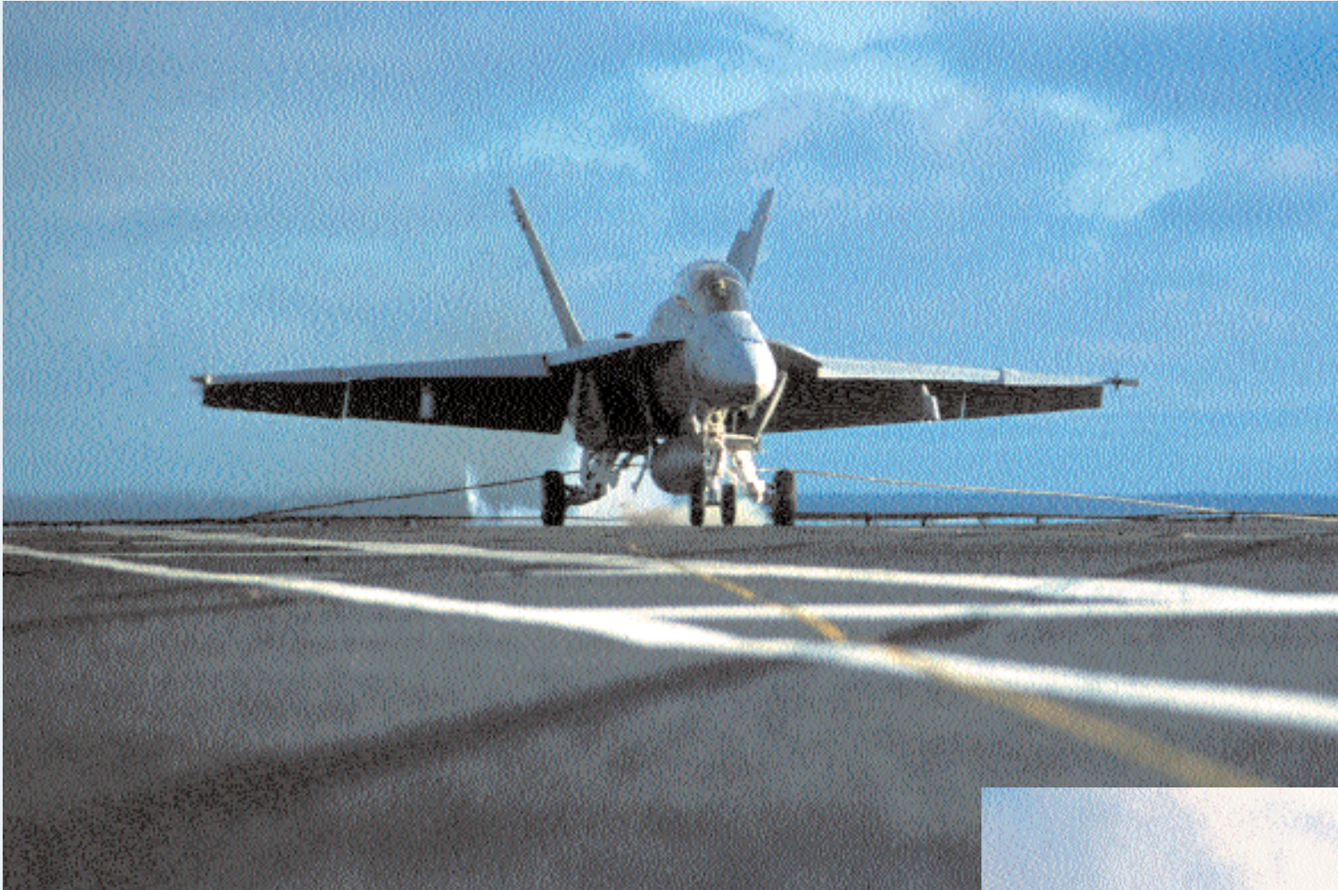
Above, a VFA-122 Super Hornet traps aboard Abraham Lincoln (CVN 72). Right, a Flying Eagles F/A-18F catches a wire. Opposite, VFA-122 instructor LCdr. Phil Poliquin will go on to a department head tour in VFA-14, one of the first fleet Tomcat squadrons to transition to the Super Hornet .
