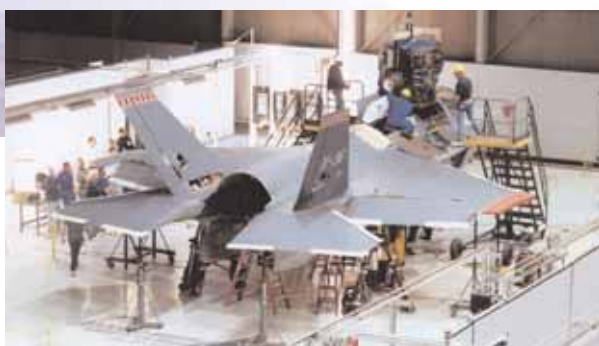
The Lockheed Martin Joint Strike Fighter prototype, above, broke the sound barrier on 21 November 2000. Left, the engine-driven lift fan is installed in the short takeoff/vertical landing version at Lockheed Martin facilities.
