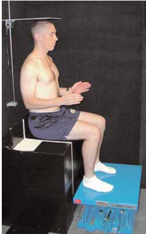
The Digital Anthropometric Video Imaging Device captures digital images of an aviation candidate in prescribed poses, above. Both the images and the physical measurements taken from them are stored in a database for future reference. Below, student aviators pore over a personality test designed by NAMRL.
