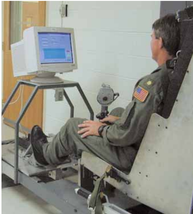
Left, a specially designed device tests a subject's ability to apply sufficient pedal and stick force.
