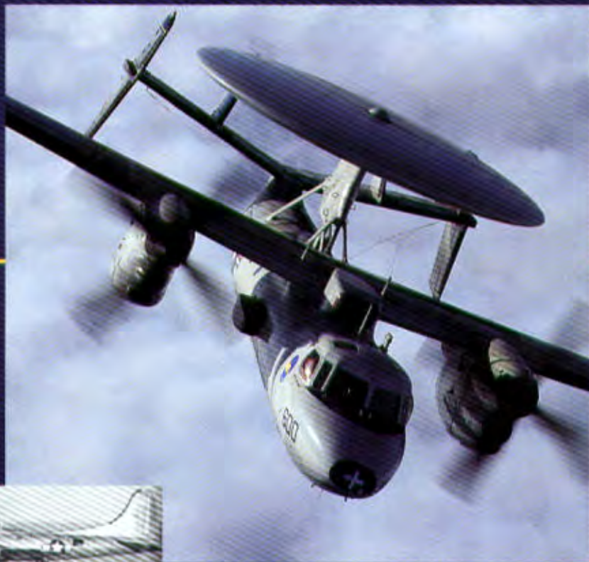
The airborne early warning system in today's E-2C Hawkeye , above, can trace its lineage back to the PB-1W, above left, a modified Army B-17G carrying the Cadillac II system and to the TBM-3W, left, which carried the Cadillac AEW system.
