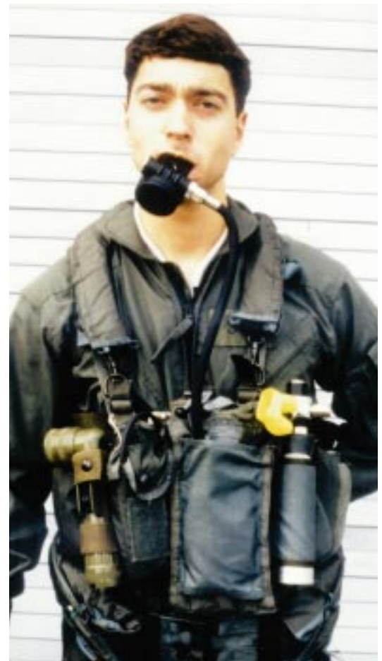
Above, the AIRSAVE flight vest will allow customized sizing and personalized pocket placement, and can be fitted with removeable armor, above right, for helicopter use. Right, the Helicopter Aircrew Breathing Device's air cylinder remains stowed in the flight vest and the user breathes through a second-stage regulator. Below, a redesigned antiexposure coverall and liner are two products of the AMELIA program, which aims to provide personal equipment that fits the physical dimensions of a wider range of users.
