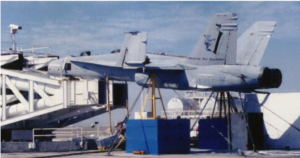
Above, V-22 aircraft #6 is prepared for testing to support the requirements of the Live Fire Test law passed by Congress in 1987. Left and below, F/A-18 state-of-the-art fire detection and extinguishing systems undergo testing under in-flight airflow conditions.
