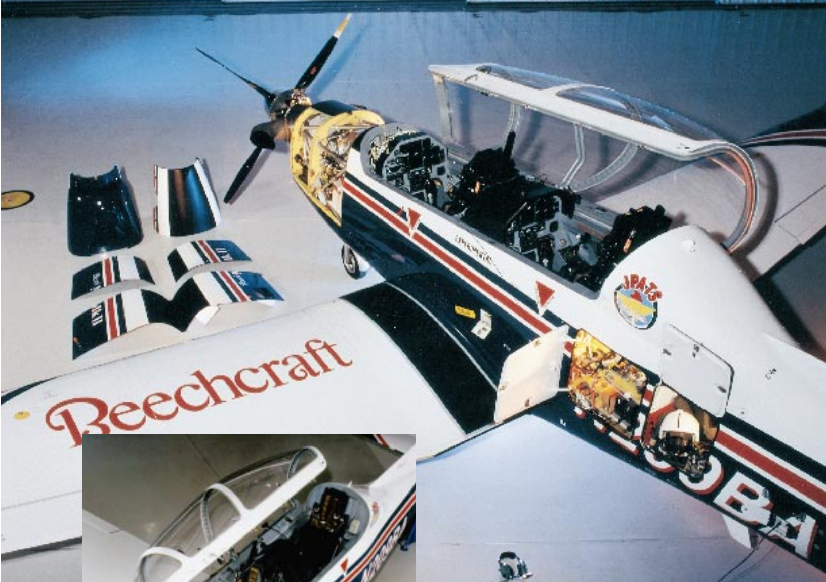
Above, the T-6A is designed for ease of maintenance. Left, safety features include Martin-Baker ejection seats and a canopy that provides enhanced bird-strike protection.
