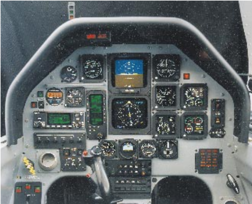
The Texan II's instrument panel features digital, liquid crystal displays, with mechanical backups of major elements.
