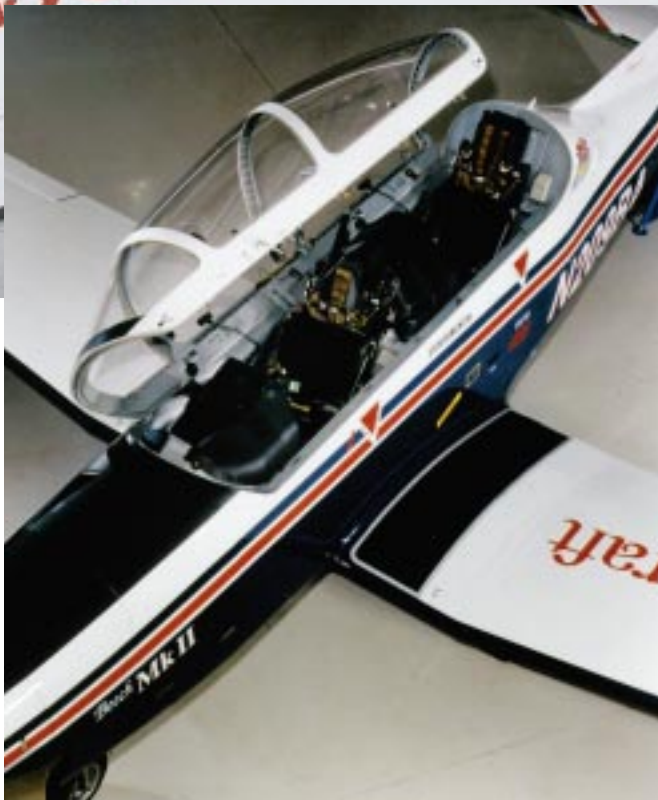
Above, the T-6A is designed for ease of maintenance. Left, safety features include Martin-Baker ejection seats and a canopy that provides enhanced bird-strike protection.
