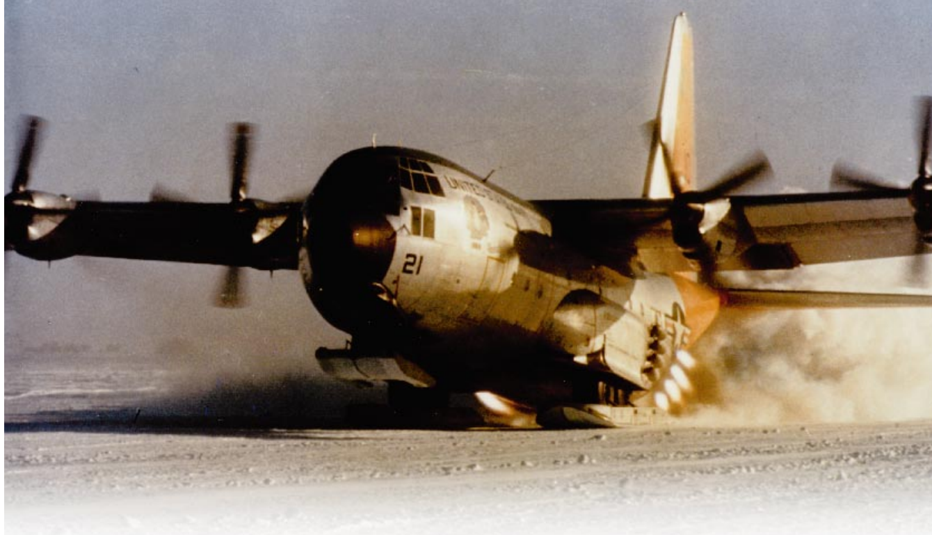
Top, jet-assisted takeoff bottles help move this ski-equipped LC-130 Hercules along the icy runway for launch. Right, a New York Air National Guard LC-130 parked near its VXE-6 counterpart in Christchurch symbolizes the changing of the guard. Below, a memorial plaque honors the 50 Americans who died in Antarctica during Operation Deep Freeze.
