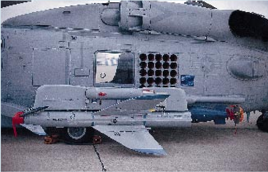
Left, this port-side view of an SH-60B shows the sonobuoy launcher and a Penguin missile mounted on the weapons pylon, two elements of the Seahawk's detection and defense system. The SH-60B's crew typically consists of a pilot and airborne tactical officer (below) and a sensor operator (bottom), with a second sensor operator on board for search and rescue operations. Opposite, landing on the platform aboard a small surface warship can be a challenge, especially in heavy seas or at night.
