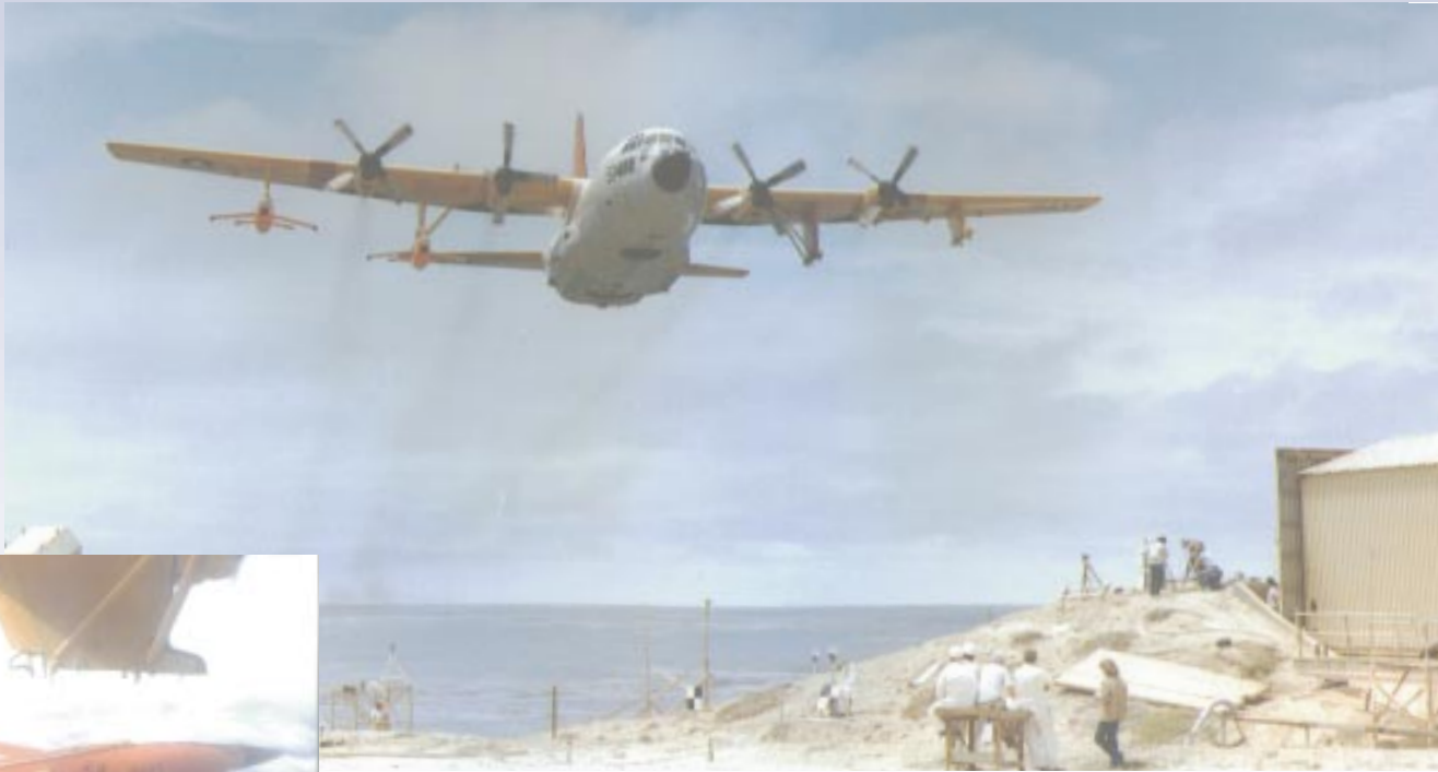
A typical missile exercise begins as a DC-130A Hercules lifts off with a pair of BQM-34S Firebee target drones (above). The crew then releases the drones (left) over the sea range. And if the drone survives the exercise, it descends to earth for recovery (below).
