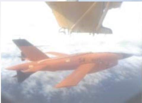
A typical missile exercise begins as a DC-130A Hercules lifts off with a pair of BQM-34S Firebee target drones (above). The crew then releases the drones (left) over the sea range. And if the drone survives the exercise, it descends to earth for recovery (below).
