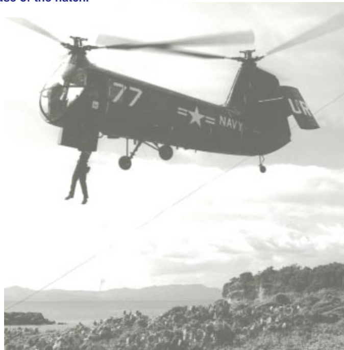
Below right, HUP-1. At the right forward end of the cabin was a unique feature of the HUP: a two-by-four-foot floor hatch opening downward through which an internal hydraulic hoist could pick up personnel and cargo, or load stretchers. The copilot's seat was folded up to enable use of the hatch.
