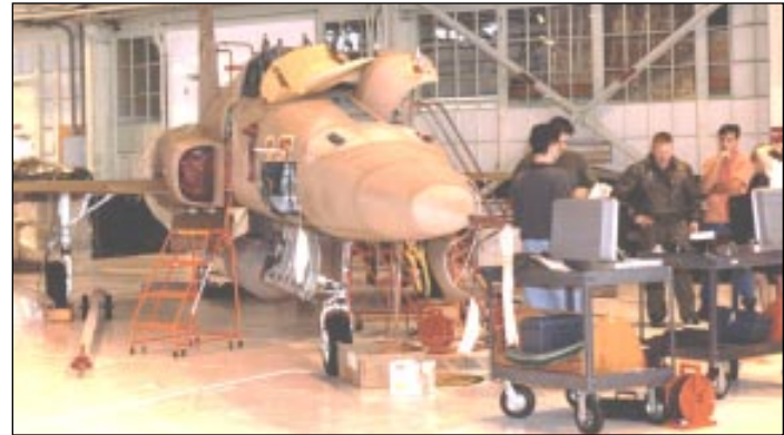
This Tiger II was instrumented for structural flight tests at NAS Patuxent River, Md.
