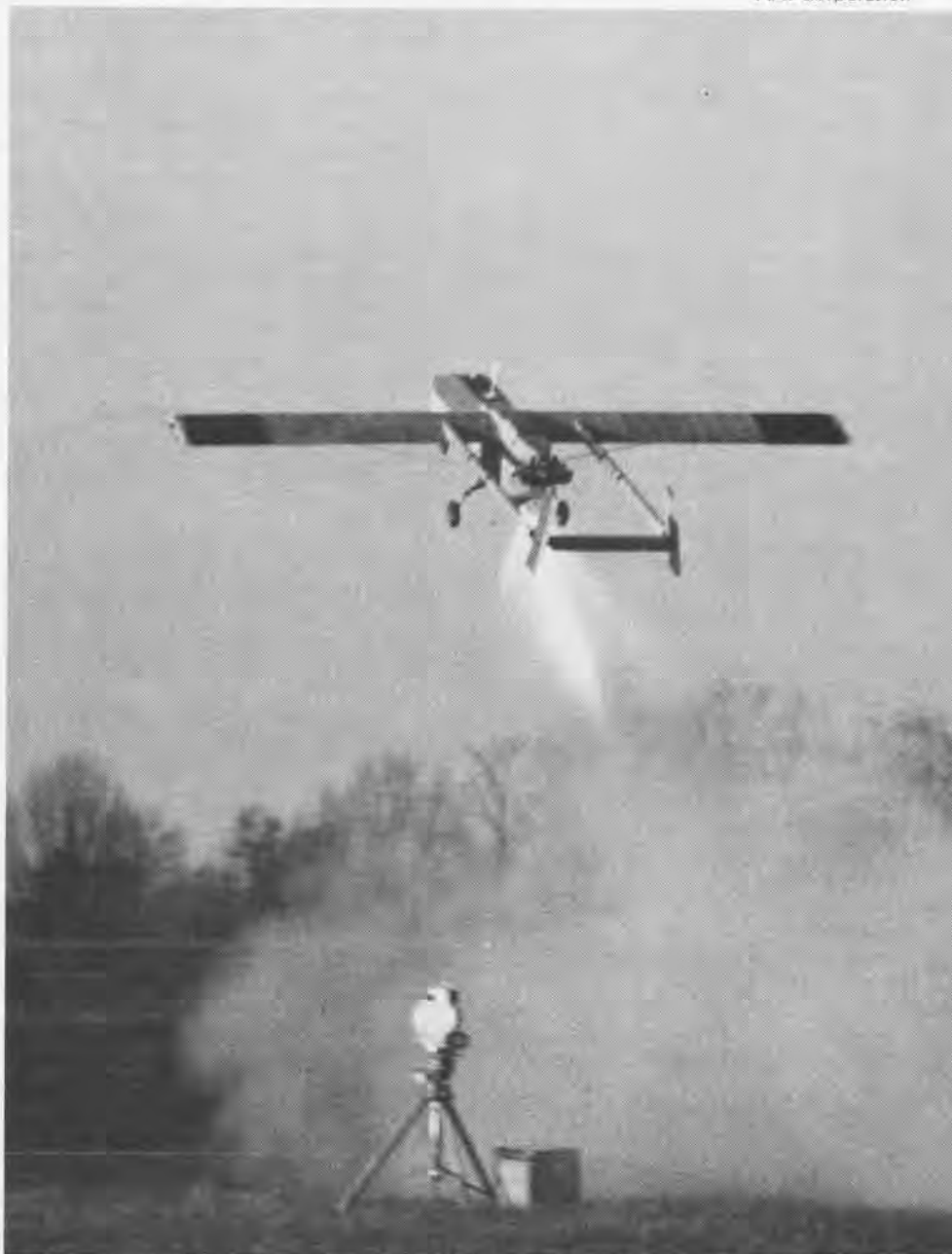
A rocket-assisted takeoff boosts a Pioneer RPV to an altitude of 160 feet and airspeed of 80 knots within two seconds.
