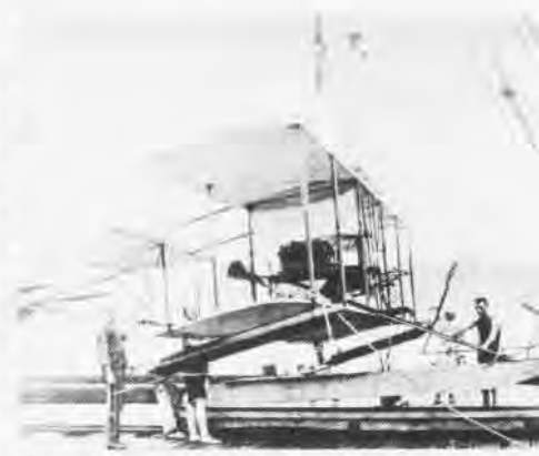
The Curtiss seaplane being placed on the catapault launching car on the Santee dock at the U.S. Naval Academy in 1912.
