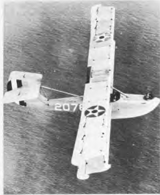
HS-2, above, was powered by a 400-hp. Liberty engine. It carried a crew of three, a Lewis machine gun, two 165-lb. bombs and was capable of four hours' flight. Here it is also armed with a Davis recoilless gun which was used for antisubmarine attack. With the HS-1's 62-foot span lengthened to add 800 feet, they were redesignated HS-2's, right. National insignia indicates it is post-war photograph.
