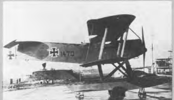
Attacks by German float planes severely limited the activity of Allied ASW aircraft in certain areas of the English Channel and North Sea. Dogfights frequently developed. Two of the more typical types were the Friedrichshafen 33L, left, and the Brandenburg W-19, right. Of interest is the unique rudder arrangement of the latter which gave the gunner a clear field of fire rearward.
