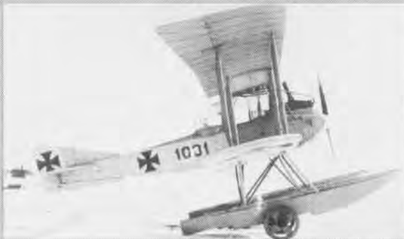
Attacks by German float planes severely limited the activity of Allied ASW aircraft in certain areas of the English Channel and North Sea. Dogfights frequently developed. Two of the more typical types were the Friedrichshafen 33L, left, and the Brandenburg W-19, right. Of interest is the unique rudder arrangement of the latter which gave the gunner a clear field of fire rearward.
