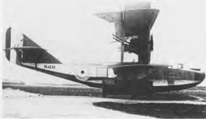
F.3, above, was almost indistinguishable from F.2A; both were developed from the Curtiss H-12. Powered by two 375 hp. engines, it cruised at 85 mph with an endurance of up to nine hours. Armament included four Lewis machine guns and bombs.
