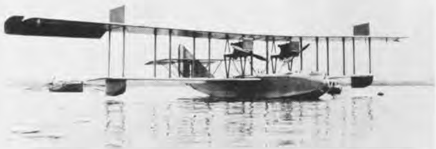
F-5L, developed late in the war from British F.5, carried 1,300 lbs. of ordnance and had greater range than the H-16. Two 200-hp. Liberty engines gave maximum speed of 102 mph.
