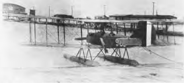
The R-9 closely resembled the R-6, including the Curtiss power plant. These planes spent many hours patrolling U.S. waters and made several attacks on U-boats. Note the unusual bomb release system.
