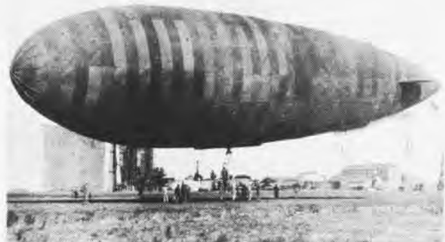
This Zodiac-Vedette was received by U.S. forces at the time NAS Paimboeuf was commissioned in March 1918. In left background is the French designed canvas hangar used for maintenance.
