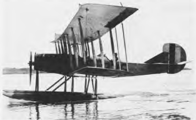
R-6's, designed as scouts, provided bulk of aircraft assigned to the First Marine Aeronautical Company at Ponta Delgada, Azores. This Curtiss-designed plane had a 200-hp. Curtiss V 2-3 engine.
