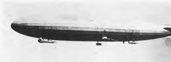
The German lead in LTA is evident by comparing the L-30, above, with those below. It had an endurance of 30 hours, speed of 63 mph, was powered by six 240-hp. engines and had 64,000-lb. payload.
