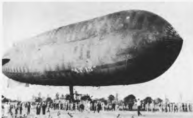
French-built Astra-Torres had two 170 hp. engines and 10-hour endurance if not operated at top speed of 50 mph. The first of these tri-lobe non-rigids was transferred to the Navy in 1918.
