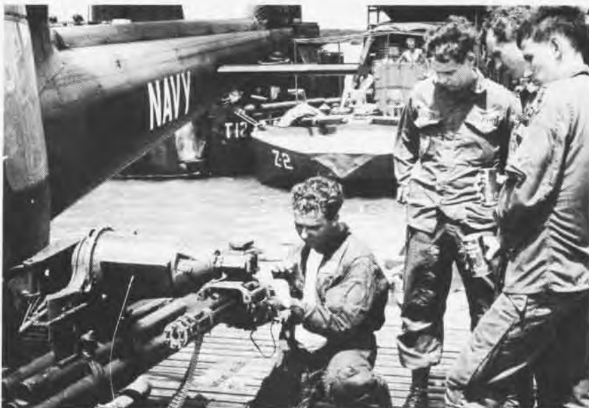
Army aviation pilots observe ADJ2 Jim Piccolo make adjustments to an M-134 mini-gun at a floating base in the Mekong Delta. Seven tube 2.75-inch rocket launcher shares same mount.
