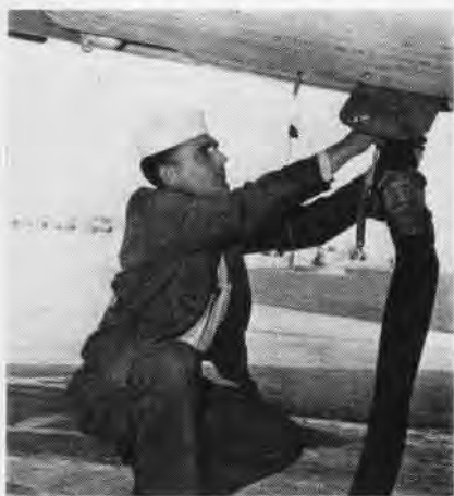
AT FUEL PIT , high pressure nozzle is connected to F3H Demon jet by A. A. Cassar, GP3.
