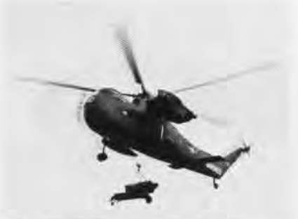
MARINE HR25 lifts XM-70, first U.S. automatic field artillery weapon, considered most significant improvement in conventional artillery since 1940. Operational by 1962, it weighs 3000 lbs., fires 12 rounds in 5 seconds.
