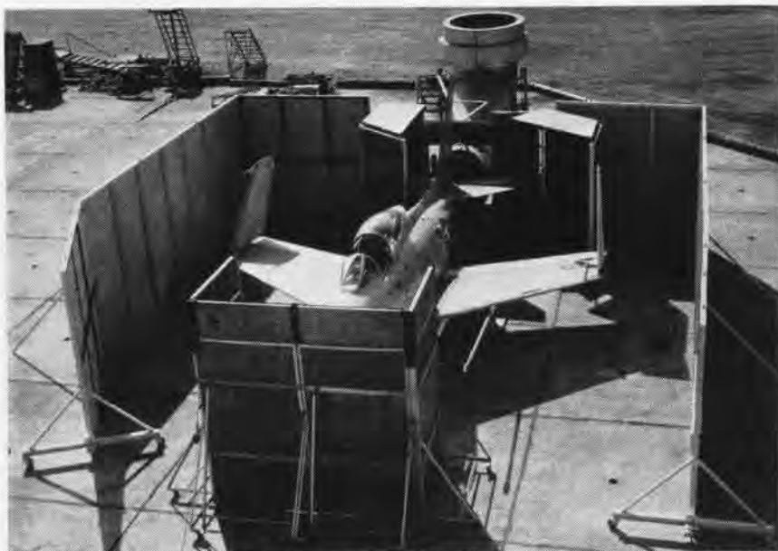
WITH SUPPRESSOR USED, THE FJ-4B FURY CAN BE RUN UP WITHOUT INTOLERABLE NOISE
