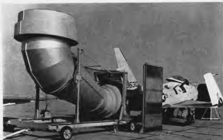
THIS PORTABLE SUPPRESSOR WAS MODIFIED AT THE NAVAL AIR STATION
