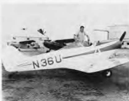
PLAYBOY, 85 hp, 18-foot single seater, with a 22-foot wingspan and a 300 mile range at 132 mph, was built by Chief Commissaryman Charles Garrison at NS San Juan. It cost about $2600 and took eight months to build.
